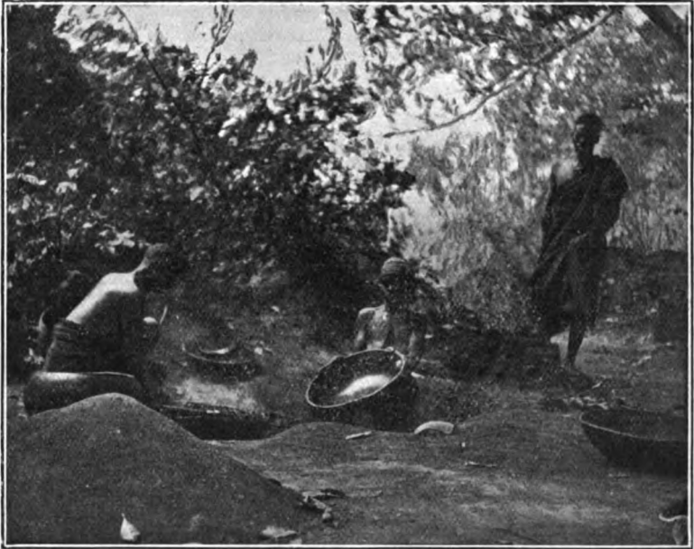
FIG. 1.—Washing the Pounded Ore.
